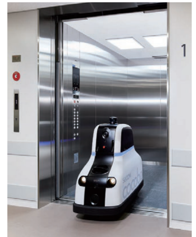
30-person passenger and freight elevator, 1st floor, South Building (Toshiba Elevator cloud service and ELCLOUD robot integration service)
