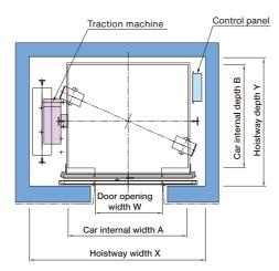
Typical floor hoistway plan (W)
