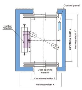
Typical floor hoistway plan (D2)
