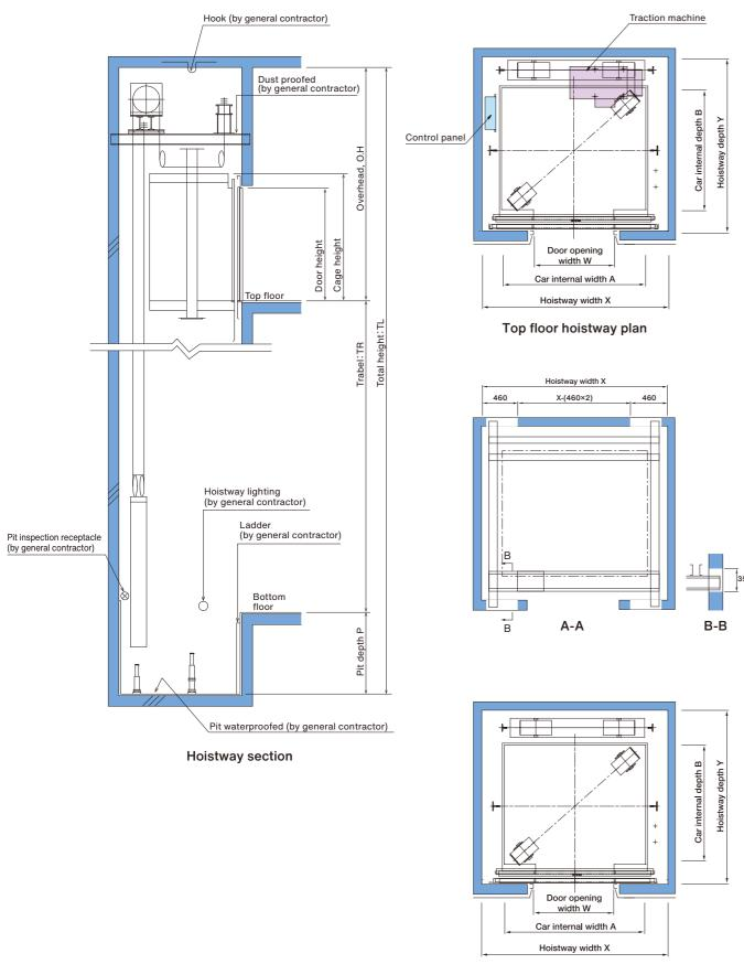
Typical floor hoistway plan
