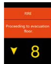
▲ Fire emergency operation
